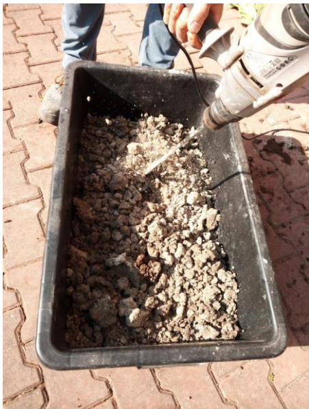
Fig. 3. Mixing of the soil with cement binder
