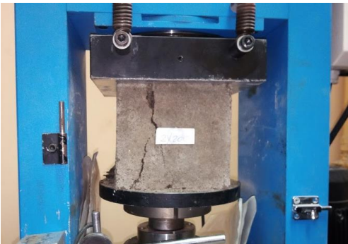
Fig. 5. Samples after compression test
