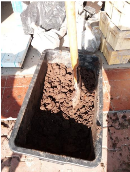
Fig. 2. Initial homogenization of the soil
