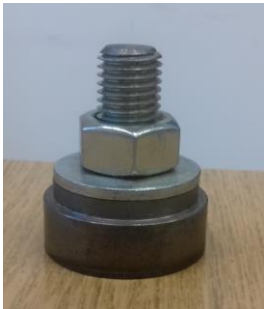
Fig. 6. Steel bottom of pile model.
