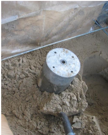
Fig. 4. Standard volume cylinder method
