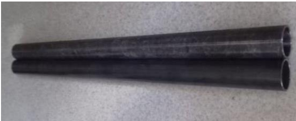
Fig. 5. Steel pipes with 40 mm external diameter
