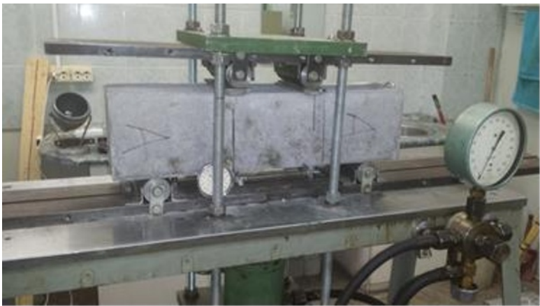
Fig. 4. Bending tensile test on samples-beams.
