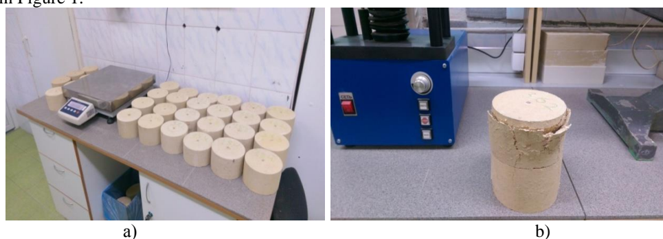
Fig. 1. Determination of the physicommechanical characteristics of the experimental samples: a) determination of average density; b) the sample after determining the compressive strength.
