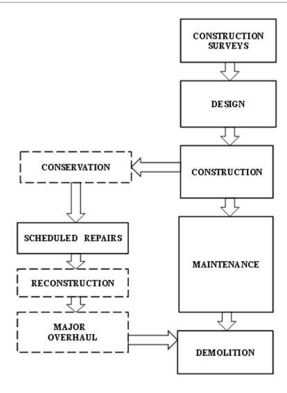
Fig. 1. Oriented structure life cycle of a construction object with mandatory stages and possible phases.
