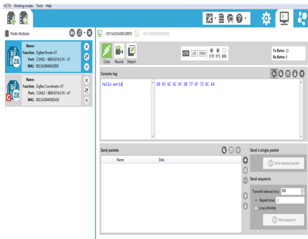
Fig.10. ‘Hello World’ written on Transmitter Console log screen.
