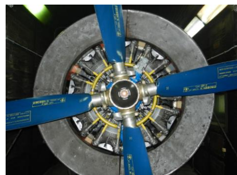
Fig. 1. Aircraft radial engine ASz-62IR - research object.
