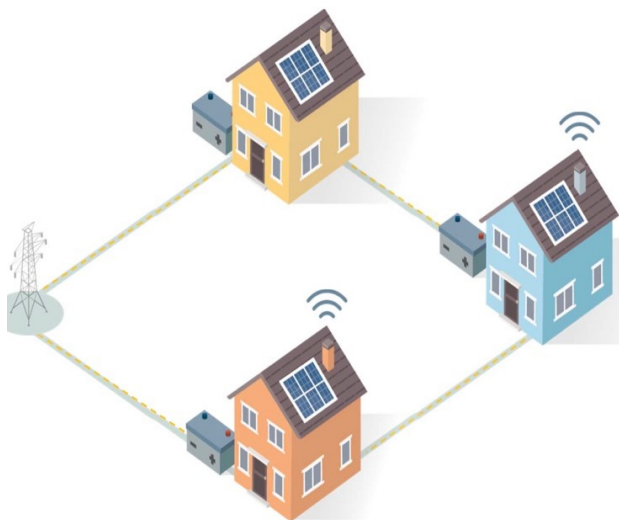
Fig. 4. SMART microgrid connected to utility grid.
