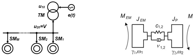
Fig. 1. An electrical diagram of the load node. Fig. 2. Non-rigid transmission of the driving pump.
