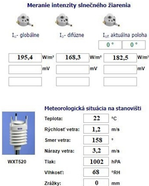
Fig. 10. Visualization of the meteorological station in the SCADA system.
