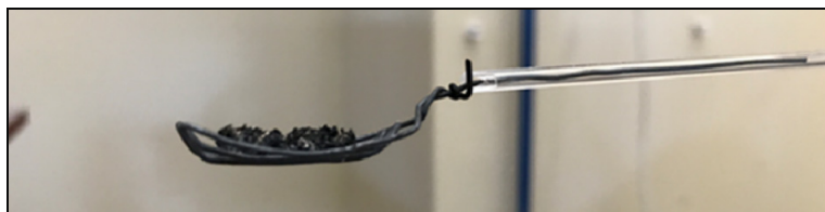
Fig. 12. The residue after combusting straw pellet at 850^\circ\text{C} , tests were carried out on the stream of inert material at G_s = 2,5\text{kg/m}^2\text{s} .
