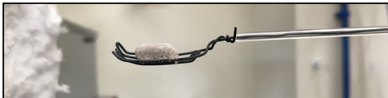
Fig. 11. The residue after combusting sunflower husk pellet at 850^\circ\text{C} , tests were carried out on the stream of inert material at G_s = 2,5\text{kg/m}^2\text{s} .
