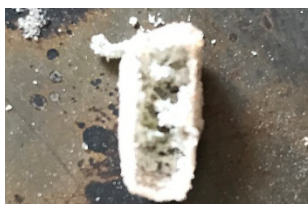
Fig. 18. Residue after combusting sunflower husk pellets at 850°C and G_s = 5 \text{ kg/m}^2\text{s} .
