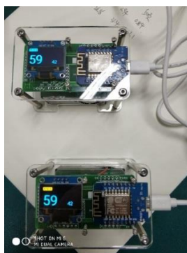
Figure 1. Laser sensor for PM2.5 monitoring
