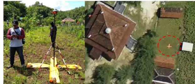
Fig. 2. The pre-marks for UAV photography, as appeared on the ground (left) and in the aerial photo (right).
