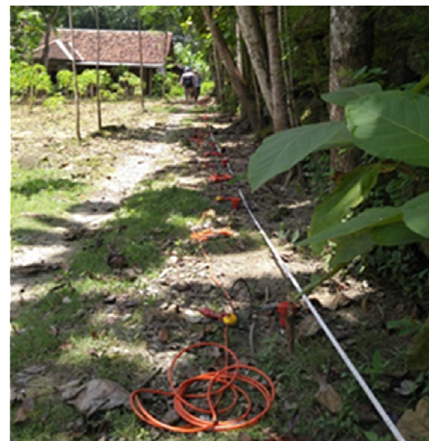
Fig. 4. Example of the geophone configuration.
