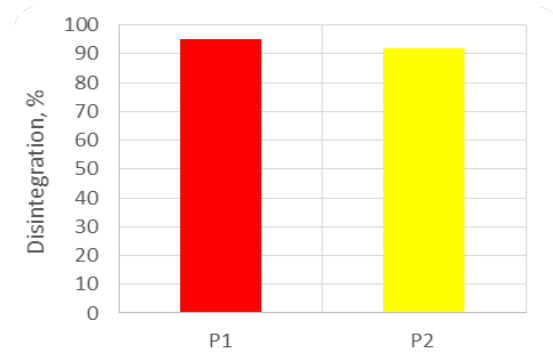
Fig. 8. Disintegration of Miocene shale sample influenced by studied mud.
