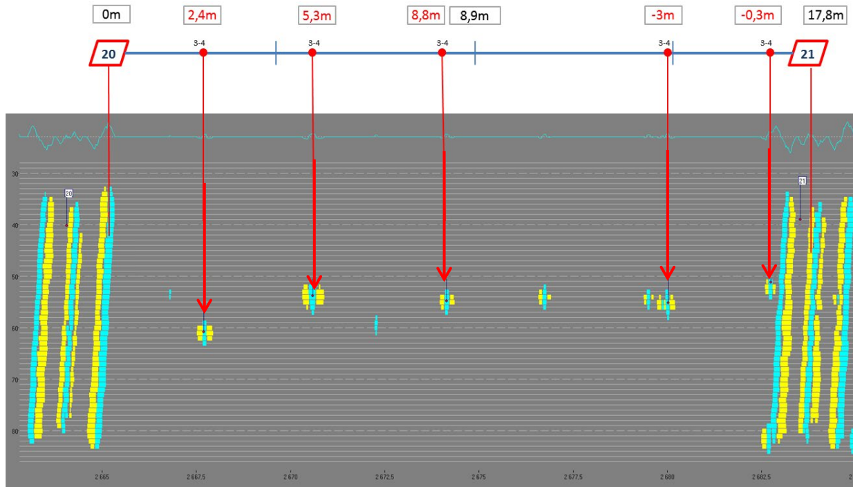
Fig. 4. A view of one of the belt’s sections with an actual defect indicated.
