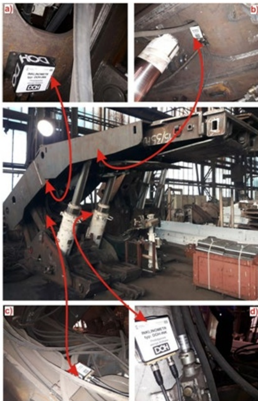
Fig. 4. Arrangement of DOH-INK prototype inclinometers on the ZRP-15/35-POz section model.
