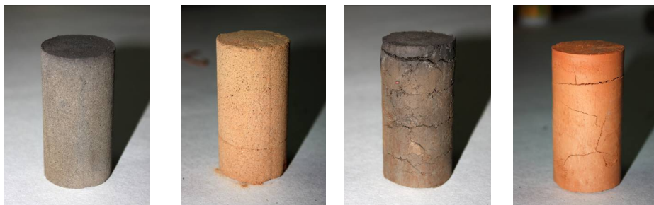
Fig. 5. Samples of sandy deposits and argillaceous deposits of Dniprobass after 400 and 650 °C temperature field effect on rock mass.
