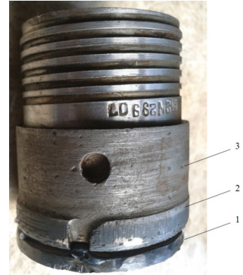
Fig. 2. Thermomechanical drill bit: 1 – friction plate; 2 – matrix; 3 – drill bit body.
