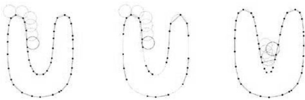
Fig. 4. The graphical representation of a structure of triangle mesh with the use of Ball Pivoting algorithm [9].
