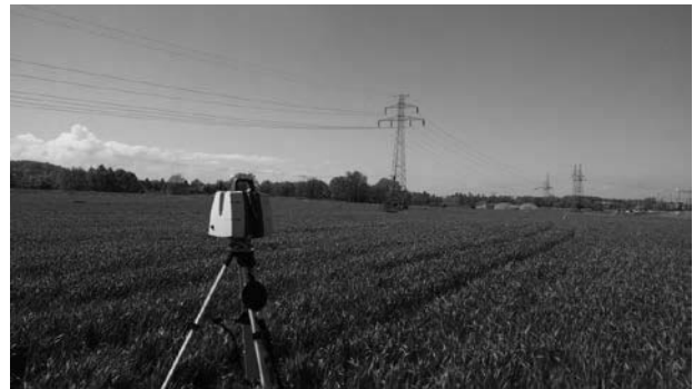
Fig. 2. The fragment of the measured power line and the set measuring instrument.
