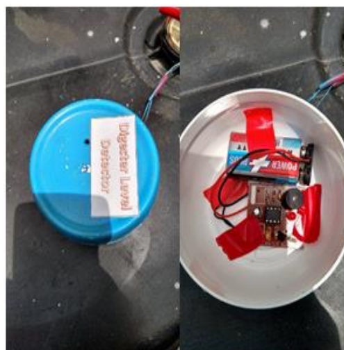
Figure 7. Digester level detector.
