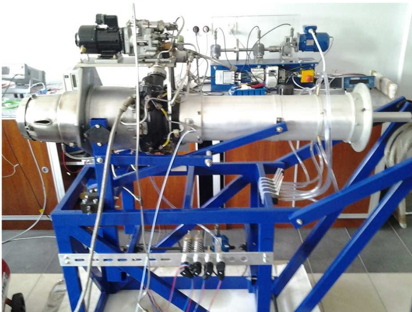
Fig. 1. The TS-21 jet engine on the lab stand
