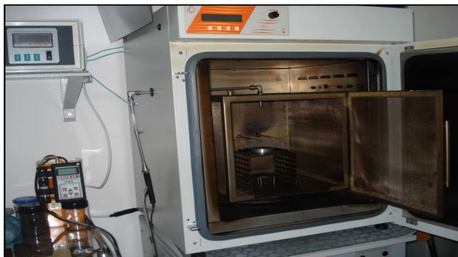
Fig. 5. Test stand for determination of the spontaneous ignition behaviour of dust accumulations (laboratories of The Main School of Fire Service)
