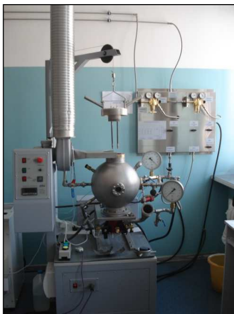
Fig. 1. Spherical test chamber of 20 dm 3 volume (laboratories of The Main School of Fire Service)
