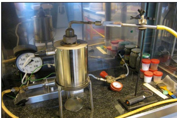
Fig. 3. Test stand (oven) for determination of minimum ignition temperature of dust cloud (laboratories of The Main School of Fire Service)
