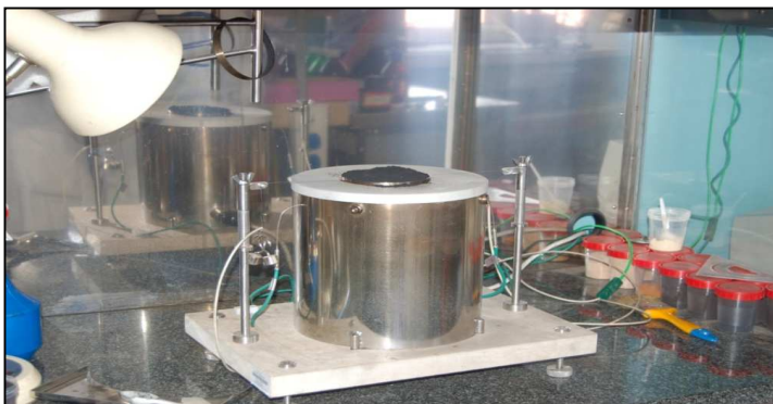
Fig. 4. Test stand for determination of minimum ignition temperature of dust layer (laboratories of The Main School of Fire Service)
