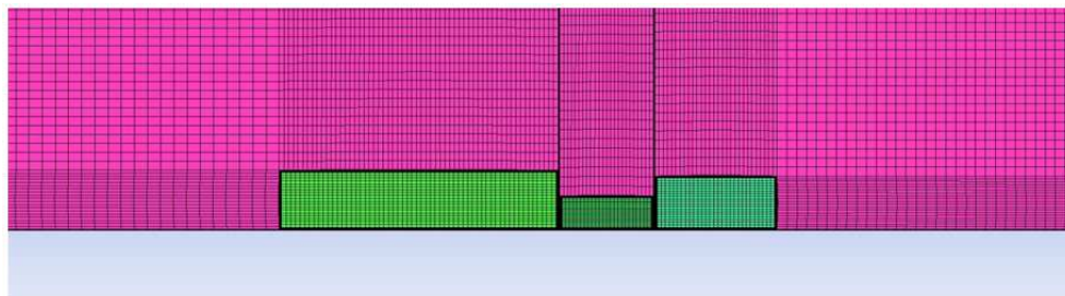
Fig. 1. Hexahedral mesh. Vehicle configuration: Truck-Car-Van and spacing 0.3m
