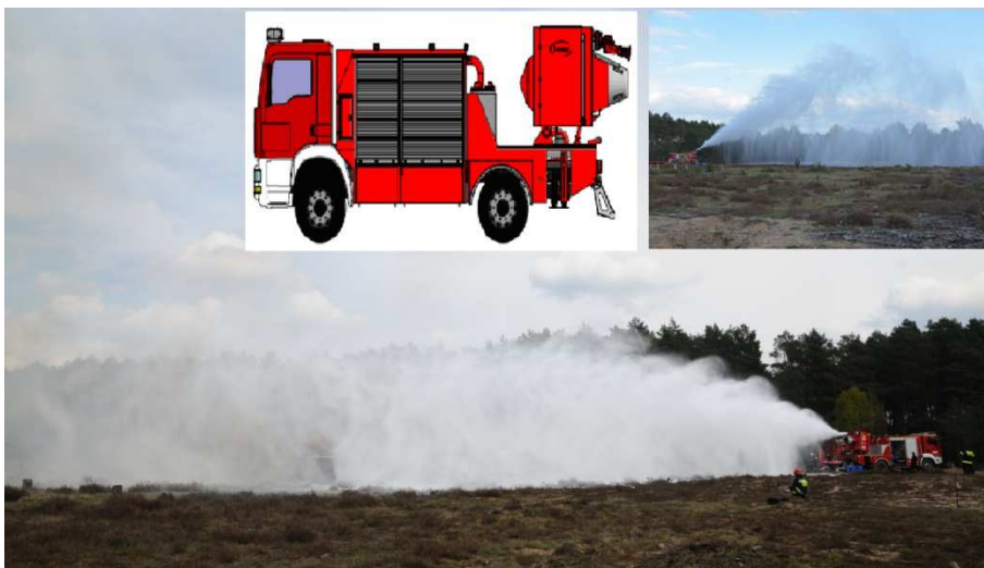
Fig. 1. Mobile turbine rescue and firefighting system (MTSRG) equipped with SO 3 -W turbine having a 10 kN thrust
