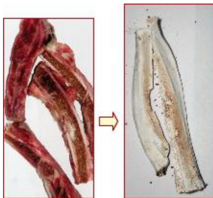
Fig. 3. Raw meat/bone substrate (100%) and product of gasification (22.6%).
