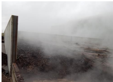
Fig. 10. Air scrubbing in a biofilter bed.
