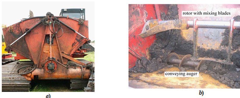
Fig. 5. Technical devices used in the machine: varying of the tilt angle of a bead (a), the mixing device and the processing screw (b).
