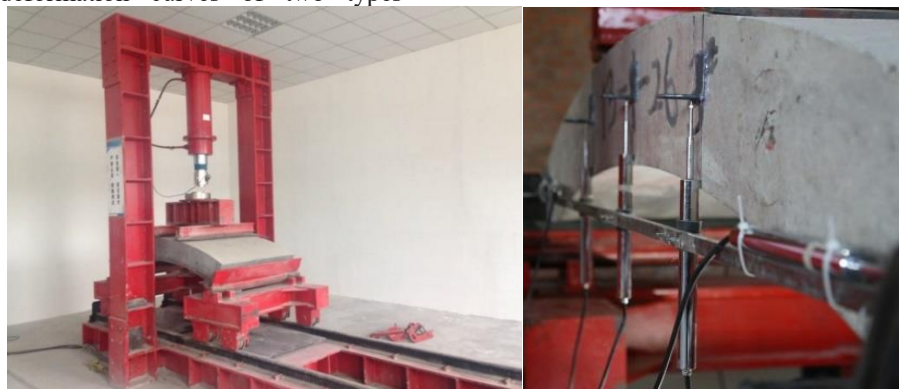
Figure 3 The segment flexural testing setup
