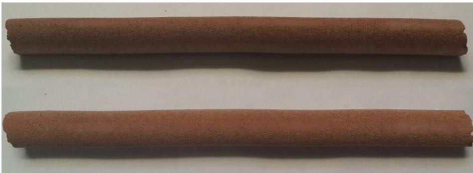
Fig. 1. A photograph of porous tubular ceramic supports.
