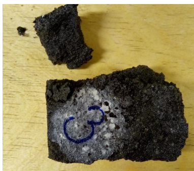
Fig 1. Mining waste sample with 5% CEM I cement + a plasticizer after the first cycles of freezing - thawing
