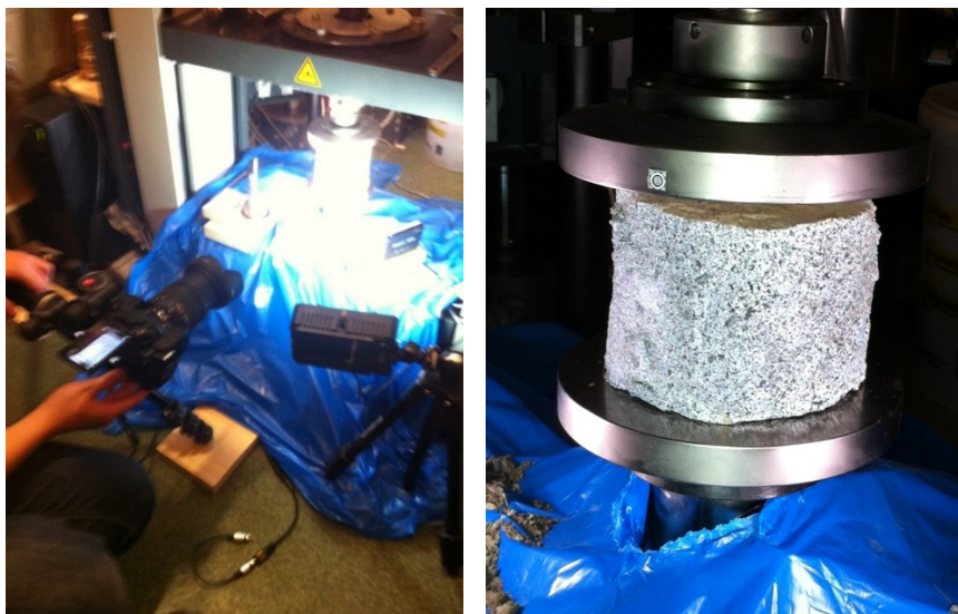
Fig. 2. The experimental setup consisting of the high resolution camera, Zwick 1455 static testing machine (left), and the soil sample tested (right).
