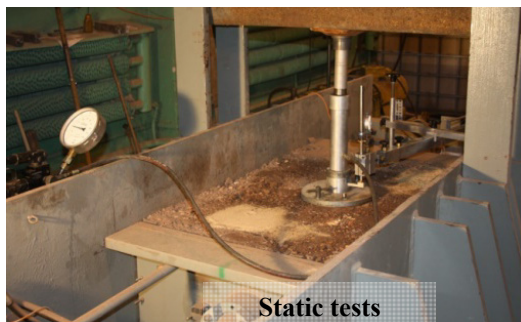
Fig. 4. The testing station during static and cyclic loading of aggregate
