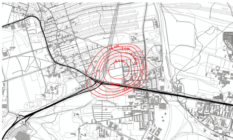
Fig. 5. Map of ground subsidence isolines that occurred between 29.11.2015 - 23.12.2015 in Bytom. Buildings located in the center of the subsidence trough were damaged as a result of underground exploitation in this area.#
