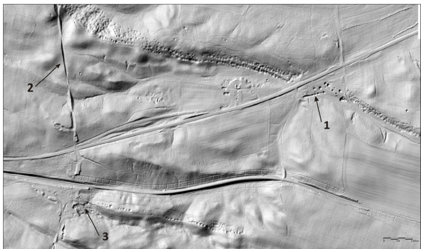
Fig. 8. A numerical terrain model of a part of the mine "Borussia" - Otto shaft. 1- descending gallery, 2 – railway between shaft and briquette factory and railway station, 3 - briquette factory
