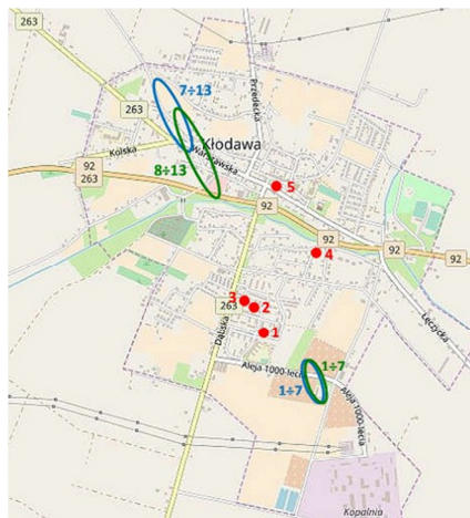
Fig. 2. Distribution of measurement detectors (red) and blasting work locations (blue: Shift I; green: Shift II). Numerals designate the blasting site according to Table 4 and 5
