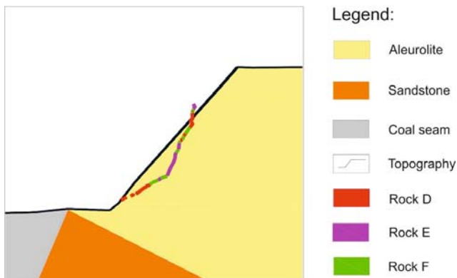
Fig. 4. Geological profile (source: geological department of Coc Sau) with profile generated from point cloud
