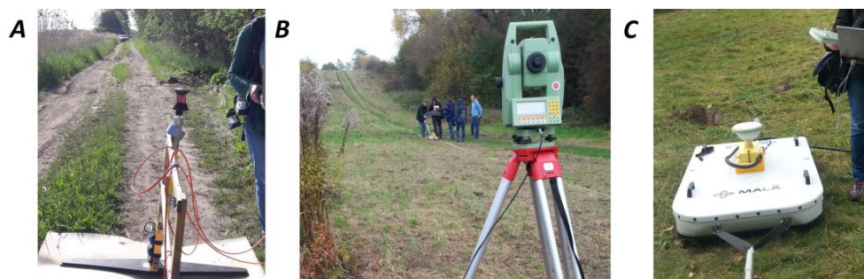
Fig. 2. Positioning systems for GPR antennas: a hip chain (A), a measurement wheel (B) and a robotic tachymeter, a measurement wheel and a GNSS receiver (C)
