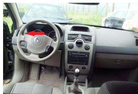
Fig. 1. Renault Megane dashboard, the considered air vent for the parametric variation of the angle of guiding vanes
