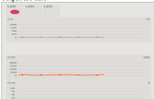
Fig 6. Measurement Results Gas CO, CO 2 and CH 4 Safe conditions
