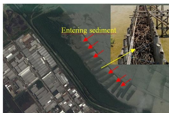
Fig. 6. Hybrid structure design to trapped sediment.
