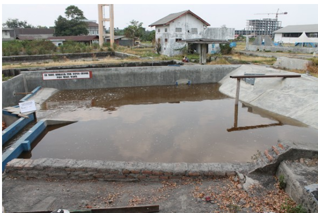
Fig. 6. Photo of Hydraulic model layout estuary leading to the reservoir with a bypass channel
