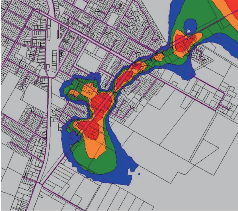
Fig. 2. Screenshot from Info Works Plus, illustrating zones with consumers of contaminated water, during the time of an incident [6].
