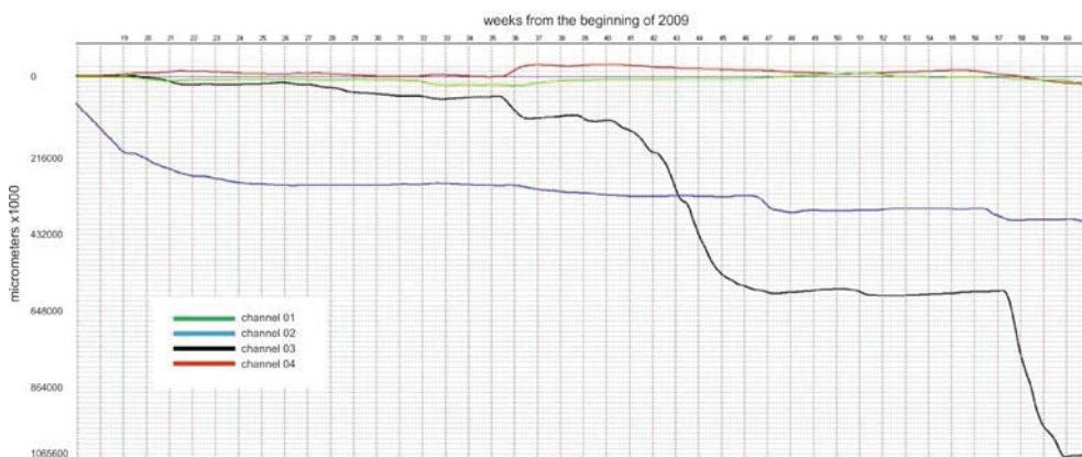
Fig. 3. Records from four measuring channels of water-tube tiltmeters from 2009.
