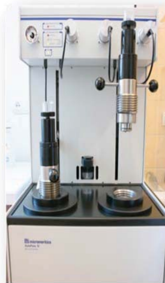
Fig. 2. Porosimeter AutoPore IV 9520 (Micromeritics) [7 , modified].
