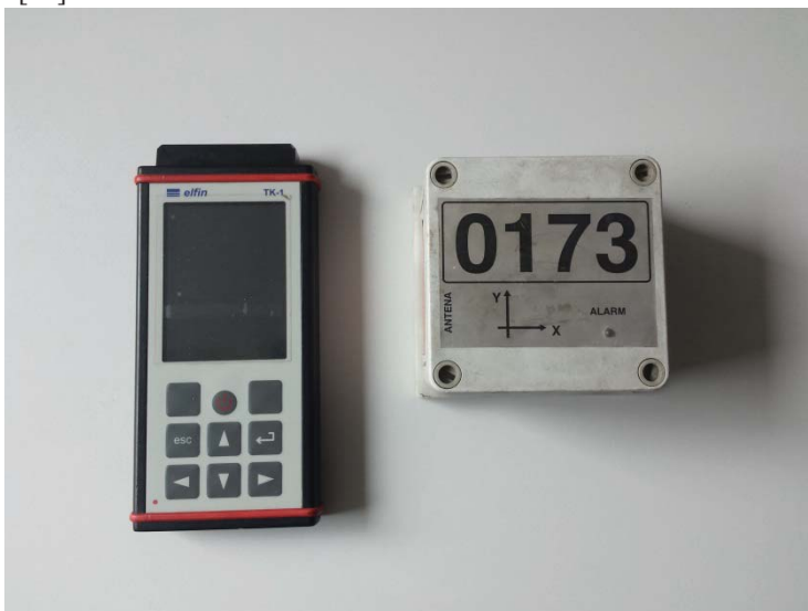
Fig. 11. Components of inclinometric measurements system: communication terminal (left) and a CNS sensor (right).
