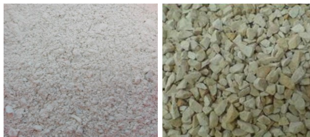
Fig. 1. Material M1 – 0-2 mm (on the left), material M2 – 2-8 mm (on the right).
