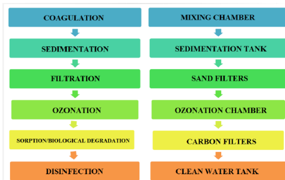
Fig. 2. Technological system used in “Mokry Dwór” Water Treatment Plant.
