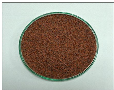
Fig. 2. Slag from the combustion of sewage sludge, fraction 800 µm.
